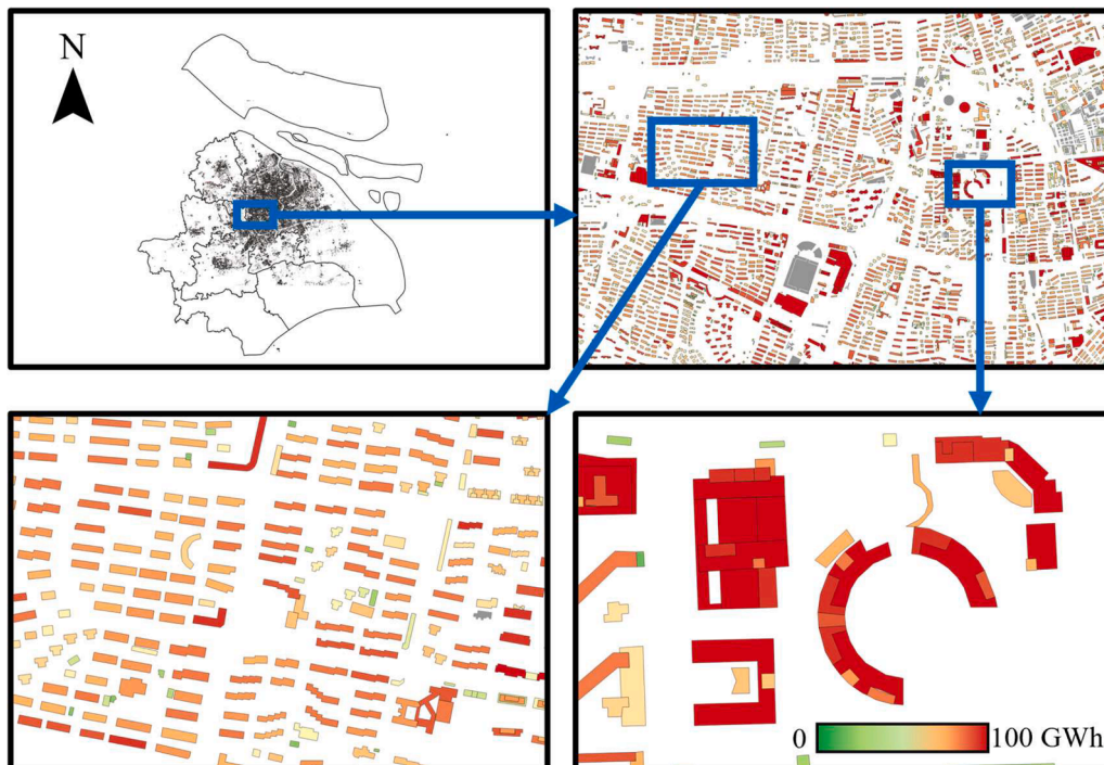
Fig. 17. Detailed building energy consumption in Shanghai.
